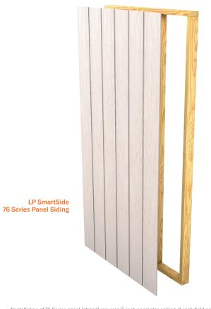
\*Installation of 76 Series panel (strand) requires 3-inch perimeter nailing, 8-inch field nailing, and application of a bead of fire caulk at vertical joints to achieve WUI compliancy.
