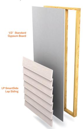
ALL: For illustration purpose only; other structural elements, insulation, plumbing, electrical wiring and finish materials not shown for clarity.
